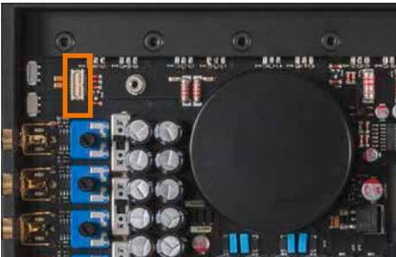
6. Insert the Allen screw which is delivered with the HDM 2 into the mounting hole of the module and fix it carefully.
